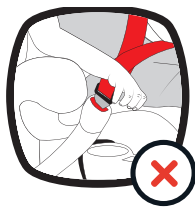
INCORRECT SEAT BUCKLE POSITION
