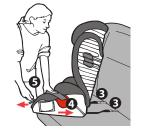
NOTE: Even with LATCH properly attached and adjusted, child seat will still have movement against the vehicle seat back and bottom
