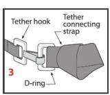
Now, use metal 'D' ring as an anchorage point for top tether metal hook.
