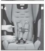
Push on restraint to force it into vehicle seat while pulling loose end of seat belt to remove slack and tighten lap portion of seat belt. (Fig. 5)
