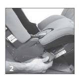
Push restraint down firmly into vehicle seat while adjusting seat belt length. Tighten and lock seat belt according to vehicle owner's manual. (Fig. 3)
