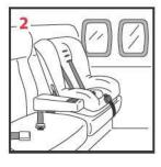
This restraint is FAA certified for use in an aircraft only as a harnessed restraint. This restraint is NOT certified for use in an aircraft as a belt-positioning booster.
